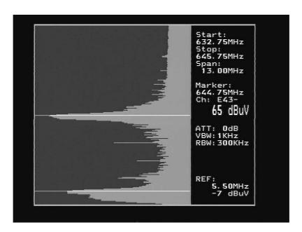
This measurement can also be made from Spectrum samples saved in memory. After a spectrum is loaded from memory with "Memory -> Load" choose" Ref mrkr" and use the knob and set the first marker position with "Ref set" and then use the knob to define the second reference marker.
