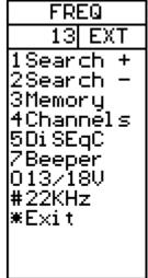
**Search +/-)** A signal search can be initiated by using the keypad '1 Search +' to search with increasing frequency or '2 Search -' with decreasing frequency. The search mode moves to the next peak in the spectrum and attempts a lock for DVB-S QPSK, DVB-S2 QPSK and DVB-S2 8PSK signals. The symbol rate is determined automatically. Because the time to lock for low symbol rate signals increases the lower the symbol rate, symbol rate signals below about 16000 will not lock during a search.
