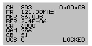
The CB value is the number of corrected bytes since lock. The UCB value is the number of uncorrected blocks since lock.
