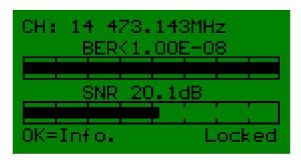
Hopefully, but not always, the digital readout; BER (bit error rate) and SNR (signal noise ratio) will correspond well with the analog setting of the antenna.
