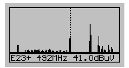
The meter shows the frequency spectrum of 48-860 MHz. A marker can select a certain channel (with the "UP", "DOWN" buttons). Signallevel (in dBuV) of that channel will be shown in the display also.
