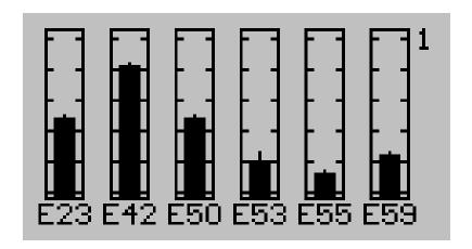
The display shows six channels on each page and there are five pages. Step through the pages with the "UP" and "DOWN" buttons.
