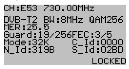
CH = The selected channel (measured at) and frequency.
