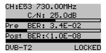
For DVB-T/T2 it can be said that, hopefully but not always, the digital readout; BER (bit error rate) and C/N (Carrier/Noise) will correspond well with the analog setting of the antenna.
