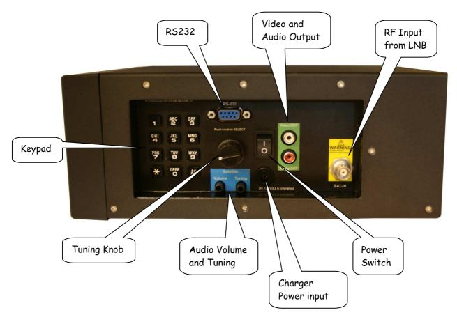
**Power Switch)** On battery power, this turns the instrument on and off. When the charger is connected, the instrument will charge with the switch off, and operate when on. The instrument will not charge when operating.
