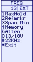
**Memory)** Samples of spectrum data can be saved in memory and then either displayed or mixed with the current spectrum. When the mix function is chosen, the current spectrum is adjusted to the same span and starting frequency, and then the spectrum from memory is overlayed as a line image so that you can compare the current signal with a saved spectrum.
