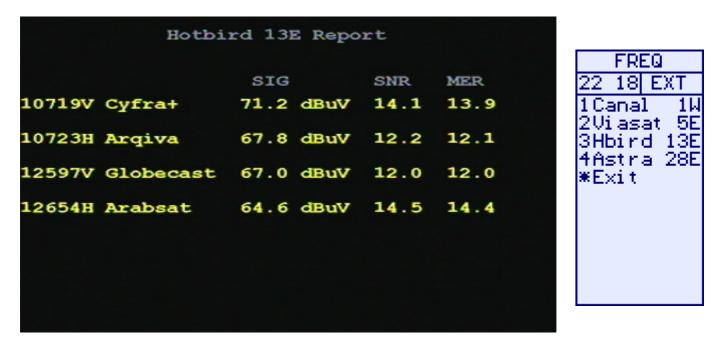
For each transponder the frequency and name are displayed with the Signal Level, SNR, and MER values. The signal level is displayed in the units chosen in the setup menu (using Setup -> Display -> Units) and can be either dBuV, dBm, or dBmV.
