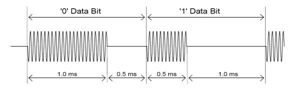
Most DiSEqC commands are 3 bytes in length but some can be up to 6 bytes long, so the transmission time of a DiSEqC message is on the order of 40 to 80 milliseconds.
