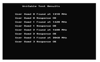
The User Band is set to 1 by default, but for more detailed testing it can be set to any of the four bands, for Example: Spec -> UniCable -> UsrBand 4. Now User Band 4 will be used for any further UniCable Tuning.
