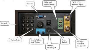
Power Switch) On battery power, this turns the instrument on and off. When the charger is connected, the instrument will charge with the switch off, and operate when on. The instrument will not charge when operating.
