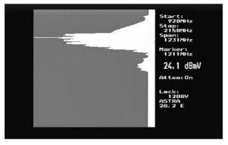
Remember that the displayed SatCR band is reflected in frequency about the User Band frequency as shown in the example below. For more details see Appendix D.
