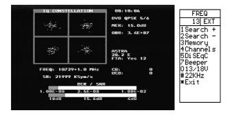
Search +/-) A signal search can be initiated by using the keypad '1 Search +' to search with increasing frequency or '2 Search -' with decreasing frequency. The search mode moves to the next peak in the spectrum and attempts a lock for DVB-S QPSK, DVB-S2 QPSK and DVB-S2 BPSK signals. The symbol rate is determined automatically. Because the time to lock for low symbol rate signals increases the lower the symbol rate, symbol rate signals below about 16000 will not lock during a search.
