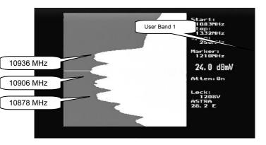
The SatCR test (Spec -> UniCable -> Uni Test) allows full testing of a SatCR LNB. This test takes about 20 seconds to check each User Band. During the test, the four User Bands are identified and any offset found is used for further SatCR tuning.
