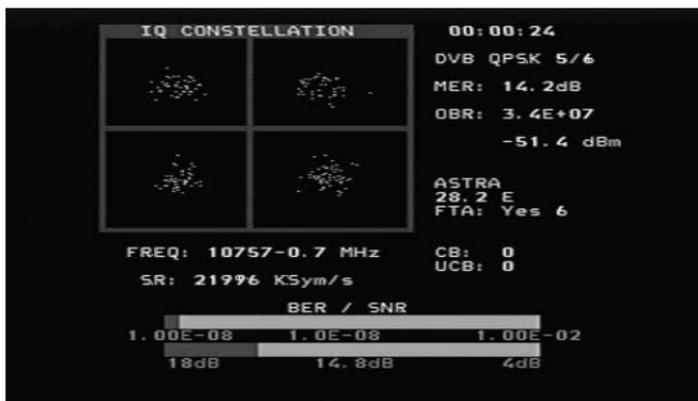
This shows a typical constellation from a DVB-S QPSK signal. The frequency and offset are shown below the constellation diagram and the measured symbol rate is shown below the frequency. The two thermometer bars show the BER and SNR of the signal. The SNR thermometer increases from right to left and the BER thermometer gets smaller from right to left, so that the best signal is shown by a longer white bar.
