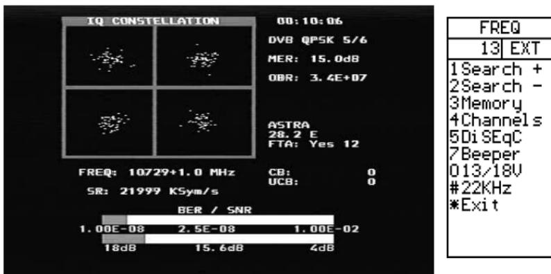
Search +/-) A signal search can be initiated by using the keypad '1 Search +' to search with increasing frequency or '2 Search -' with decreasing frequency. The search mode moves to the next peak in the spectrum and attempts a lock for DVB-S QPSK, DVB-S2 QPSK and DVB-S2 8PSK signals. The symbol rate is determined automatically. Because the time to lock for low symbol rate signals increases the lower the symbol rate, symbol rate signals below about 16000 will not lock during a search.
