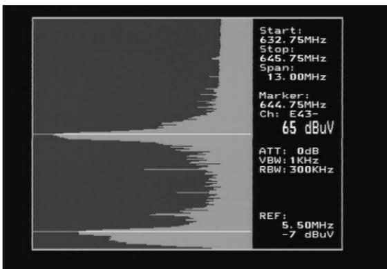
This measurement can also be made from Spectrum samples saved in memory. After a spectrum is loaded from memory with "Memory -> Load" choose "Ref mrkr" and use the knob and set the first marker position with "Ref set" and then use the knob to define the second reference marker.
