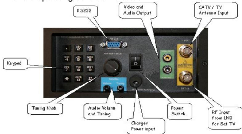
**Power Switch)** On battery power, this turns the instrument on and off. When the charger is connected, the instrument will charge with the switch off, and operate when on. The instrument will not charge when operating.
