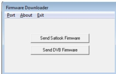
Select the RS232 port on the computer. Normally, the port is COM1 but some USB to RS232 will use some other port. If desirable, this USB to RS232 conversion device can be made to always use COM1 by clicking Control Panel / Device Manager / Ports and in the Advanced settings for the adapter set to COM1.
