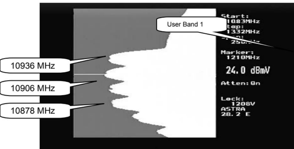
The SatCR test (Spec -> UniCable -> Uni Test) allows full testing of a SatCR LNB. This test takes about 20 seconds to check each User Band. During the test, the four User Bands are identified and any offset found is used for further SatCR tuning.
