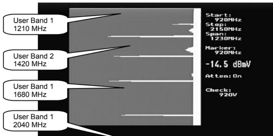
At the end of the test, the results of measuring the User Bands are presented.
