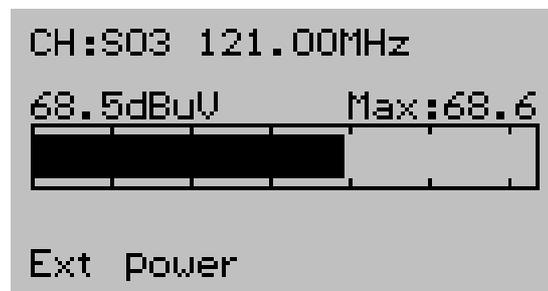
Press down the mode button again when the antenna is pointed in the right direction. This will put the meter in the **Digital-mode**.
