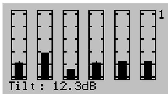
The display shows six channels on each page and there are five pages. Step through the pages with the "UP" and "DOWN" buttons. Select different view on bottom row with "OK" button.
