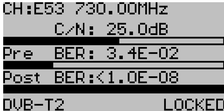
Hopefully, but not always, the digital readout; BER (bit error rate) and C/N (Carrier/Noise) will correspond well with the analog setting of the antenna. Quite often the antenna needs to be re-directed a little bit in order to maximize the digital-values (which are of more importance than the analog readout).
