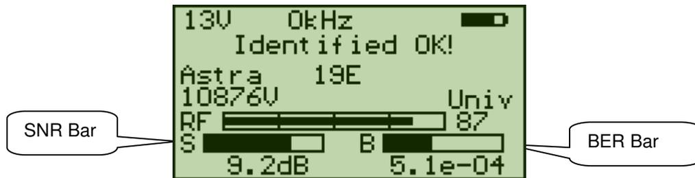
Once “Locked” on a signal, the satellite is confirmed with the MPEG data stream using the TSID and ONID (transport stream ID and Original Network ID) for the chosen transponder
