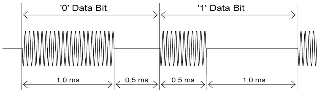
Most DiSEqC commands are 3 bytes in length but some can be up to 6 bytes long, so the transmission time of a DiSEqC message is on the order of 40 to 80 milliseconds.
