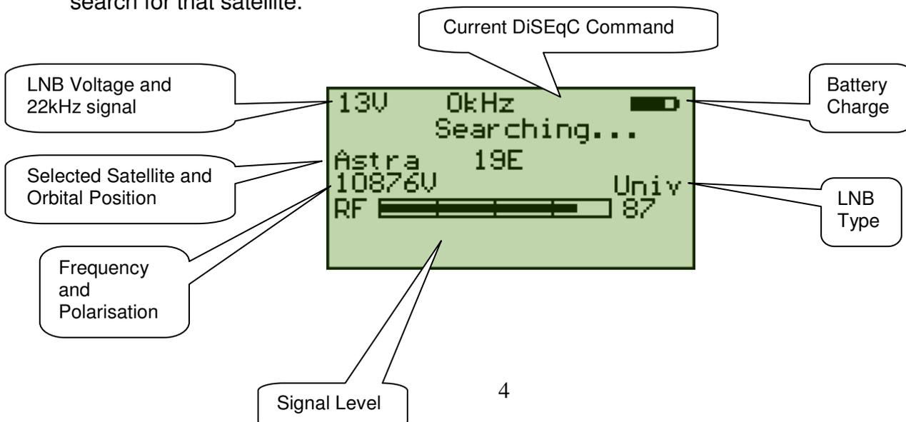
The signal level will increase on the signal bar if any satellite signal is detected. If the beeper is enabled, then the pitch of the beeper will increase with signal strength. Once the instrument locks on a satellite transponder, the display is changed to include SNR (signal to noise ratio) and BER (bit error rate) bars and numeric values.
