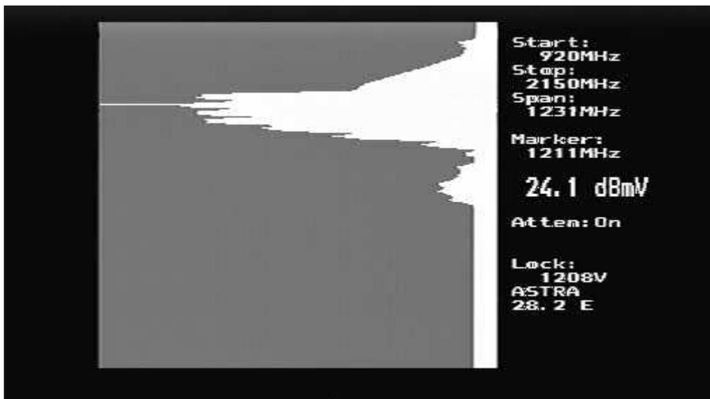
Remember that the displayed UniCable band is reflected in frequency about the User Band frequency as shown in the example below. For more details see Appendix D.
