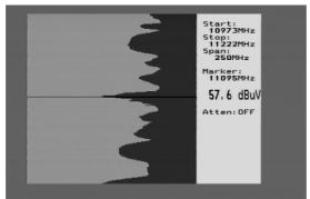
Rotate the LNB so that either the Horisontal or Vertical polarisation will be in its max-position –adjusting the **cross-polarisation**.
